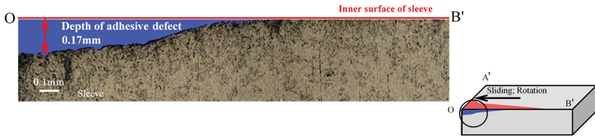
Fig. 8 Cross-sectional observation of Adhesive defect ② at OB' z=\text{const.} surface of the sleeve in Fig.5 (a)
