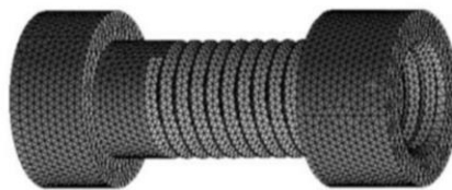
(a) FEM model M12 bolt and nut
