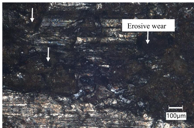
(c) Erosive wear in Area B in Region 5 of slip defect ②.
