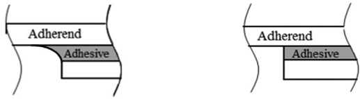
(a) With fillet (adhesive geometry in experiments) (b) Without fillet (analysis model in this study)
