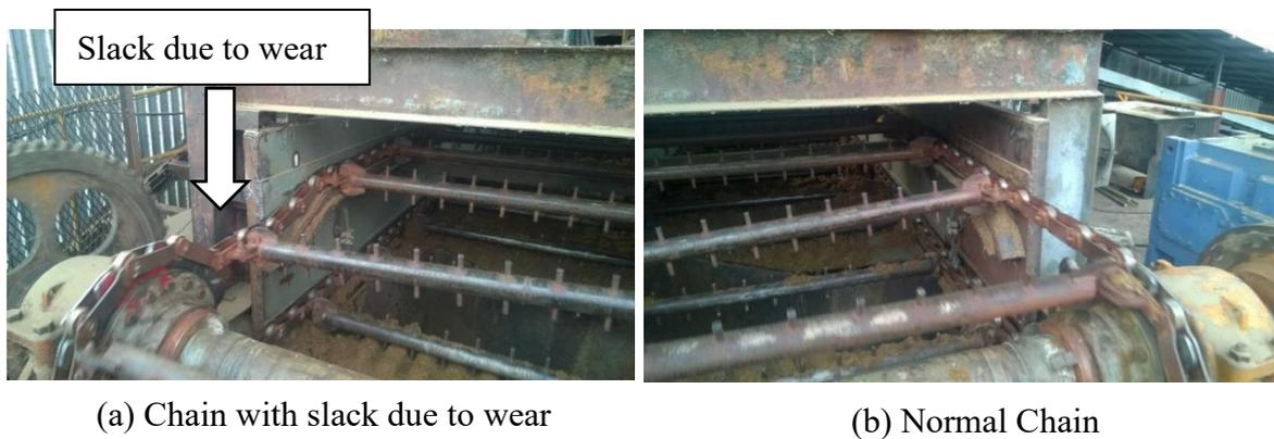
Fig. 4 Chain elongation due to wear during operation
