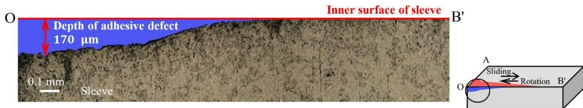
Fig. 4-13 Cross sectional observation of adhesive defect ② at the z = \text{const.} surface of the sleeve in Fig. 4-11.
