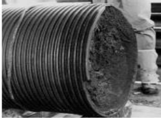
Figure 1.1: A giant bolt failed because of the fatigue fracture, 1975, Japan [2].
