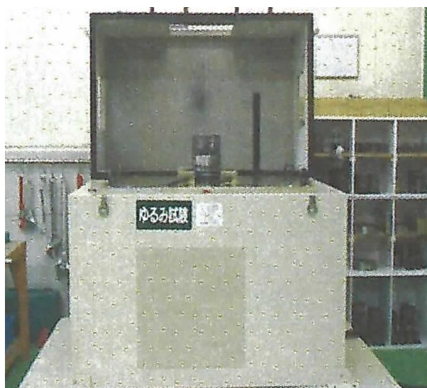
(a) Loosening experimental device
