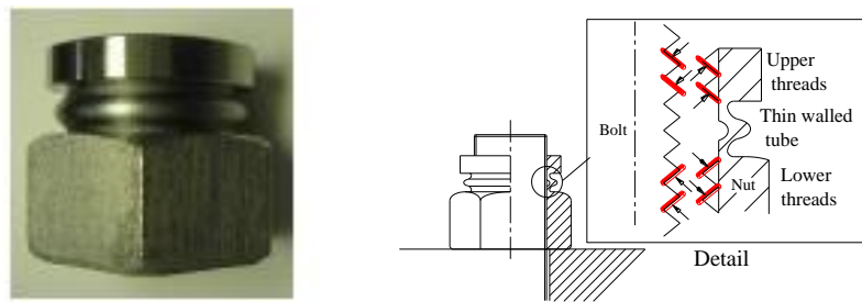
Figure 2.1: Super Lock Nut
